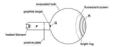
The heated filament emits slow-moving electrons.
